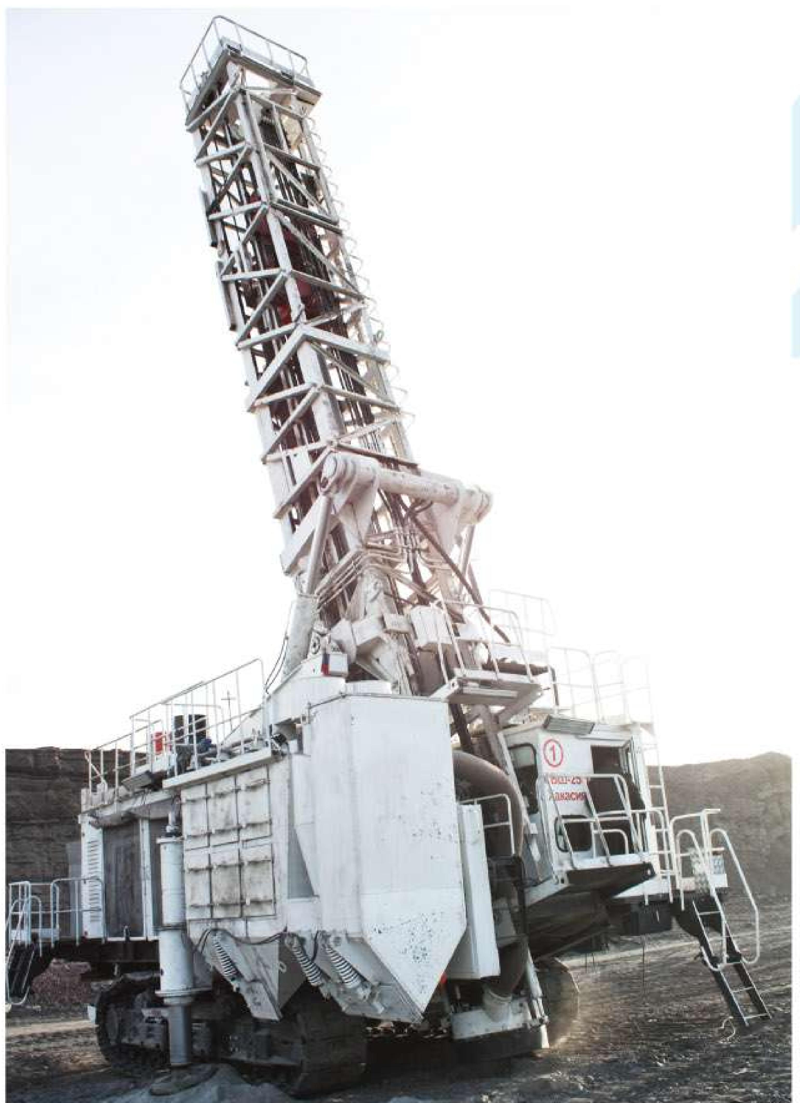
The rotary blasthole drilling rig СБШ-0250Д is specified for drilling blast holes with diameter 200-270 mm in hard highly abrasive rocks. The diesel drive provides autonomy which meaningfully decreases time and expenses for moving the drilling rig not depending on remounting the network of the quarry.
