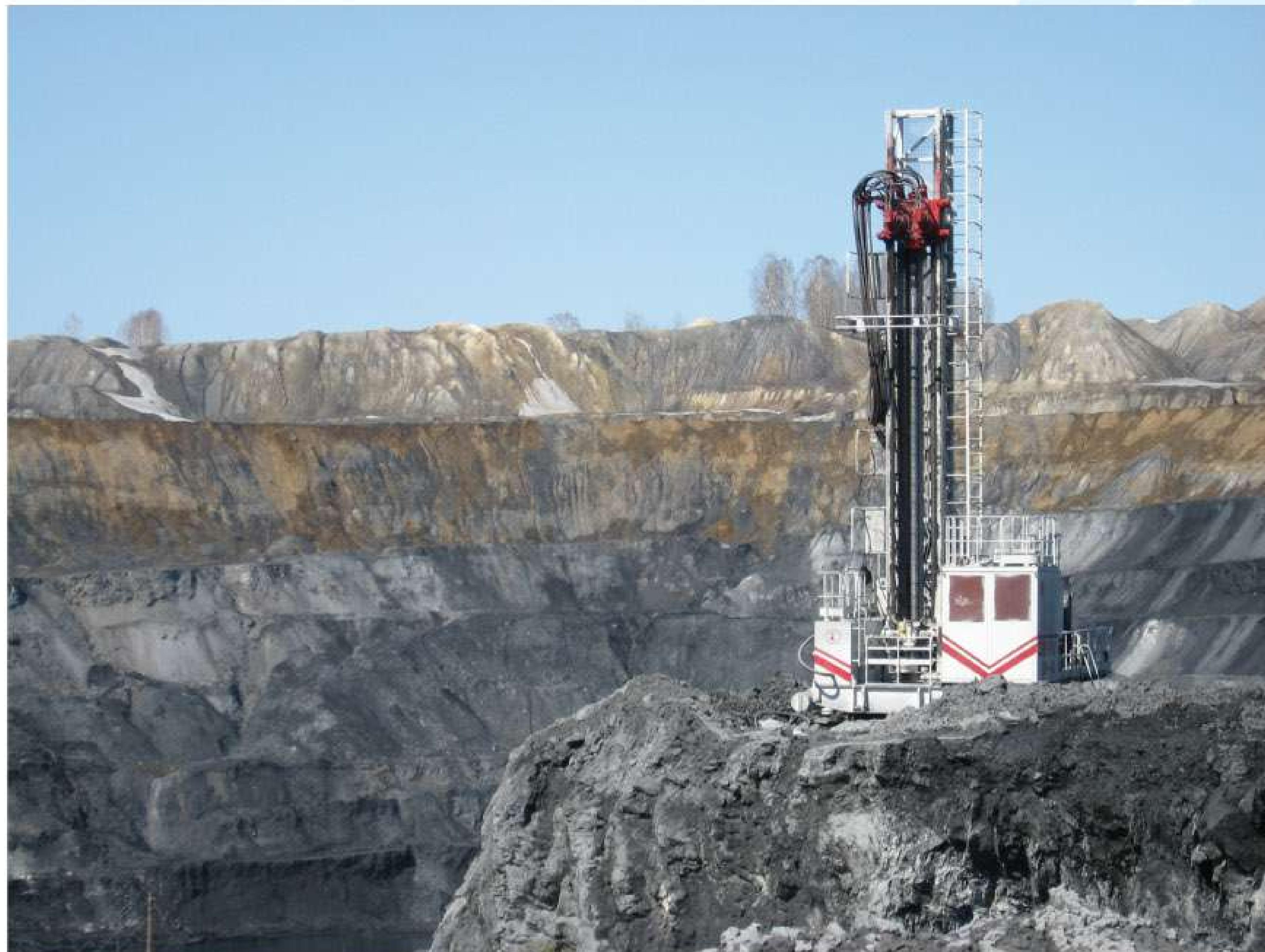
Gidrofitsirovanny, with the electric drive, the machine boring sharoshechny type is intended for drilling of technological explosive wells in breeds by fortress = 6...18 units on a scale of the prof. Protodyakonov on open-cast mountain minings of minerals, and also when working on заоткоске ledges of boards of pits on a limit contour. Components of the machine are placed on a platform which is established on a caterpillar drive of excavator type.
